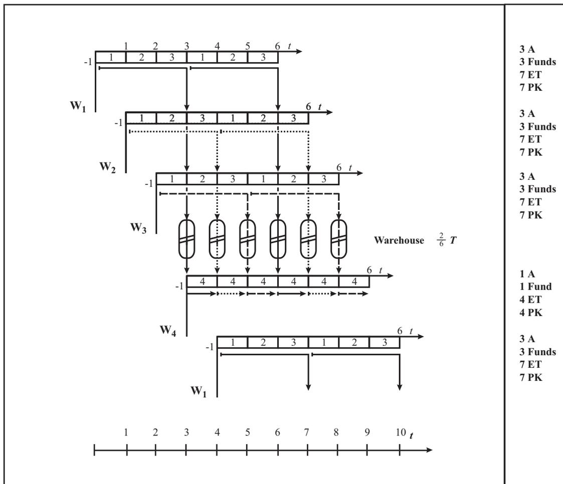
Fig. 5. Line production with idle times. Four workers and eleven elementary tasks: example a.
