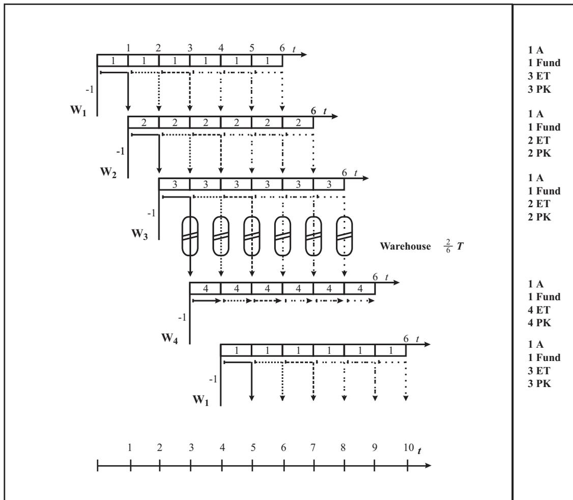
Fig. 6. Line production with idle times. Four workers and eleven tasks: example b.
